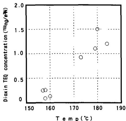
Fig.3 Effects of gas temperature on dioxins at the bag filter.
