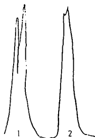
Fig. 4: Effect of HOAc concentrations on peak shape. 1. represents 1.2 g/L NaOCl, 2. represents 1.07 g/L NaOCl.
