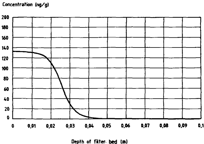
Fig. 3: PCDD- and PCDF-distribution in a 100 mm coke layer
